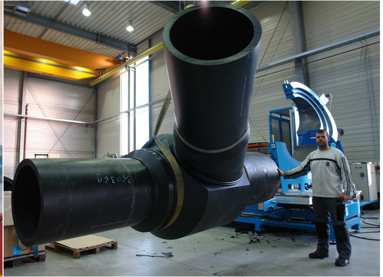
Fig. 2: PE 100 branch; 45 °; OD (800/630 mm) SDR 13.5; Service pressure 12.5 bar
