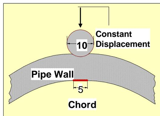
Fig. 1: Loading by an external point load before starting the internal pressure test
