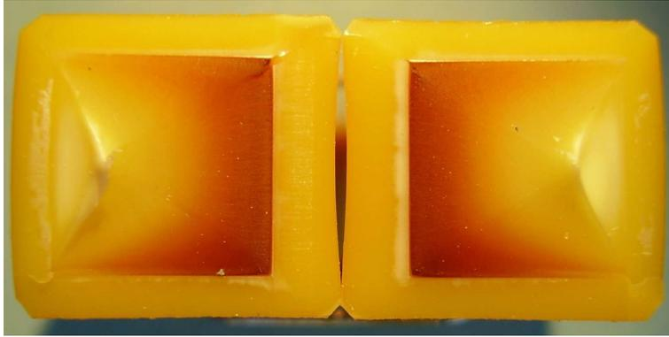
Fig. 5: Fracture surface of a FNCT-specimen taken from a PA 12-pipe (8 N/mm<sup>2</sup>)
