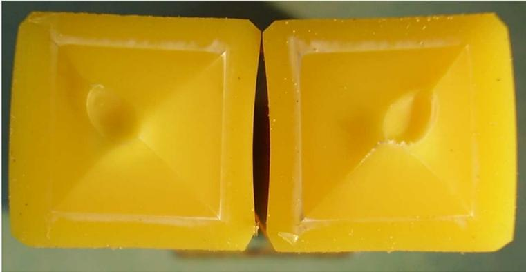
Fig. 4: Fracture surface of a FNCT-specimen taken from a PA 12-pipe (16 N/mm<sup>2</sup>)
