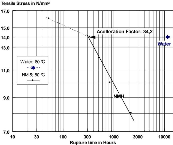
Fig. 3: Creep rupture of PA 12 in the FNCT at 80 °C
