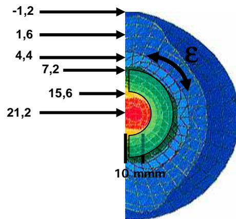
Fig. 2: Edge fiber expansion in % at the inside wall of the pipe due to an external point load and an internal pressure of 8 bar
