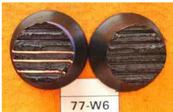
Fig.X Fracture surface of tensile creep test specimen through the plane of the heating wires.
