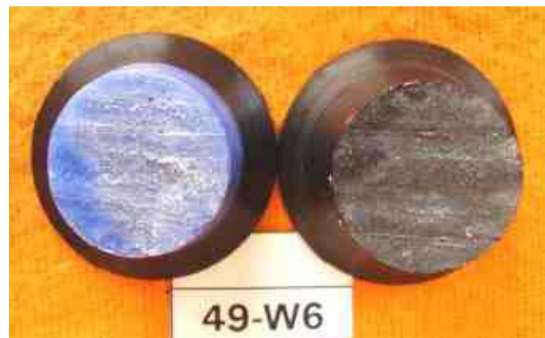
Fig.XI Fracture surface of tensile creep test specimen through the weld interface.
