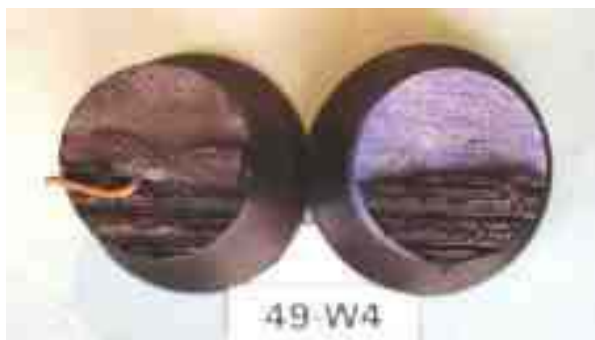
Fig.XII Fracture surface of tensile creep test specimen showing a mixed failure mode.
